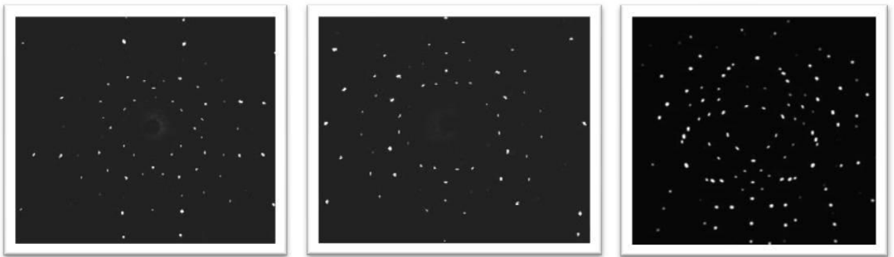
Crystal orientation of three different planes of a silicon crystal.
