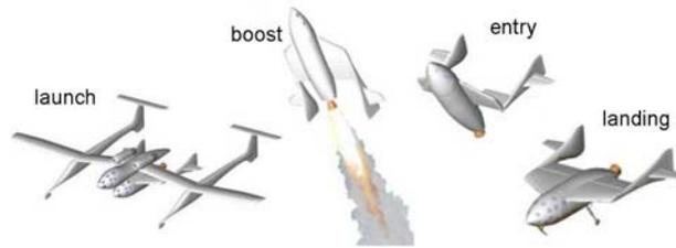
**Figure 7 SpaceShipOne Flight Configurations**
