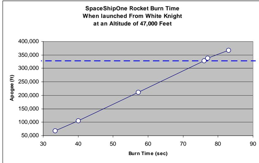
**Figure 9 Rocket Apogee versus Rocket Engine Burn Time**
