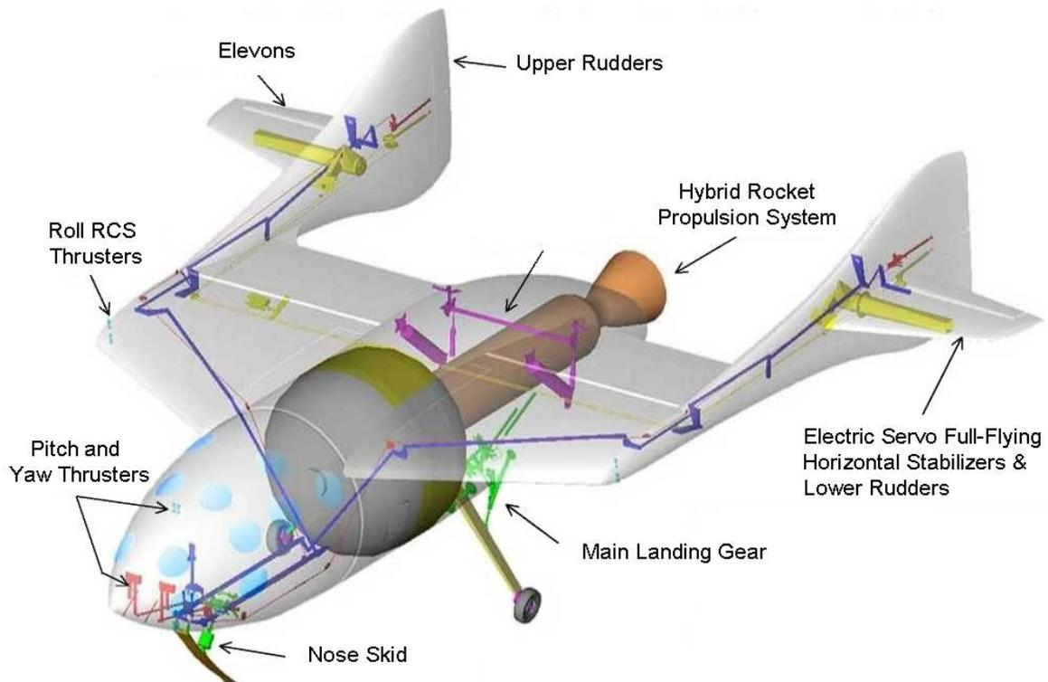
**Figure 2 SpaceShipOne Internal Systems View**
