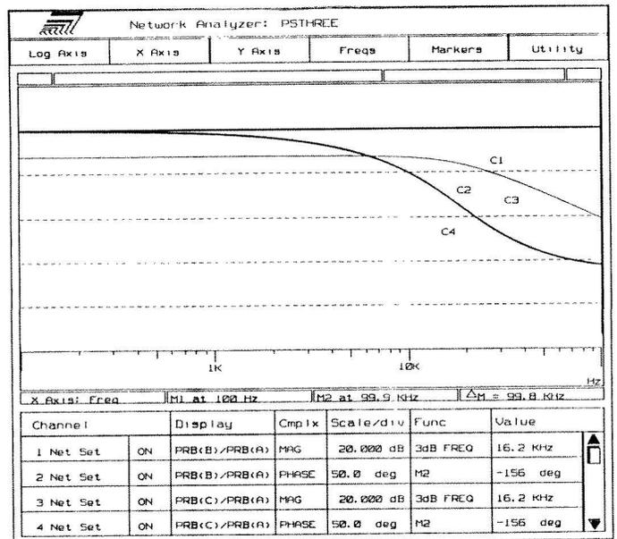
A comparison between the four topologies (state average, coupled core, uncoupled inductors and reflected inductance) shows that from a small signal stand point the state average model has the same response as the reflected inductance model and the coupled core inductor model has the same response as the uncoupled inductor model. This is shown in Figure #8.
