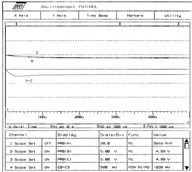
there still seems to be some high frequency error in the small signal response when comparing Figures #13 to #6. This may in part be due to the discontinuous inductor current as was present in the uncoupled state average model.
