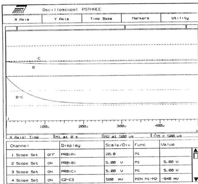
By using the PWMBCKD model the designer can also determine quite easily whether the individual inductor currents are continuous. The state average transient response shown in Figure #9 compares closely to the switching transient response shown in Figure #1. However, there still seems to be some high frequency error in the small signal response when comparing Figures #10 to #6. This may in part be due to the discontinuous inductor current.
