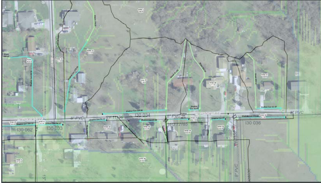
Figure 5: sheet and shallow flow classified base on area for every structure in Lincolndale
