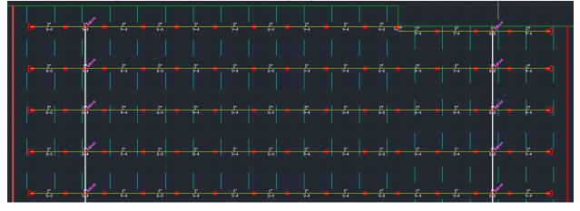
This means that for each zone split, the mains have to be placed after two heads on each side of the zone. The image above displays it. The next step is to go through the layout and place the riser nipples.
