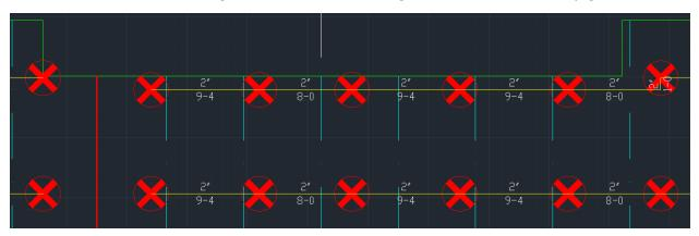
As you can see in the image above, the top lines of heads is lower around the jog but the heads are spaced using the same pattern. After I continued the pattern and placed each head, I also put in my pipe for each head.
