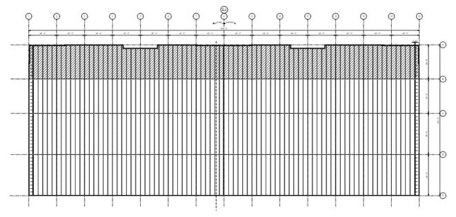
The image above shows my building size of 560'x220'. It shows my A-frame joist pattern that's running vertical from column line one through fifteen, as well as my expansion joint at column eight. Running horizontally are the girders. These are represented by column lines A through E.
