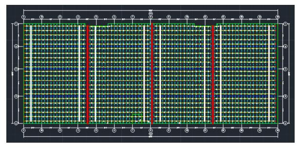
The mains are the thick, white lines running in a vertical just like the zones. This type of layout is commonly referred to as a "grid system". There is also such a thing called a "tree" system. A grid system, such as this one, requires that the two mains be only 2 sprinkler heads in on each side.
