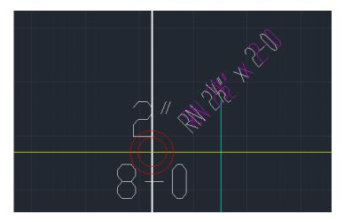
According to the NFPA-13 in 3.5.9 a riser nipple is "A vertical pipe between the cross main and branch line." These are used to supply water to our branch lines. Our mains are hung lower than the sprinkler branch lines, thus we need something that joins the main and the branch lines together. The two-and-a half inch number represents the diameter of the pipe, and the two-foot number represents the length of the pipe. The next step is to place in the water source to feed the systems.
