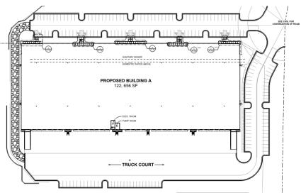
This site plan shows the basic, outer shell of the building, as well as the property layout. This is useful because it shows me where my pump room is. The pump room is where my four riser sprinkler assembly lead-ins are for the building.
