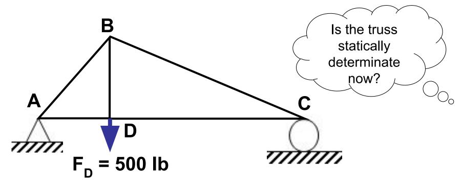
A truss is considered **statically determinate** when the static equilibrium equations can be used to find the reactions on that structure.
