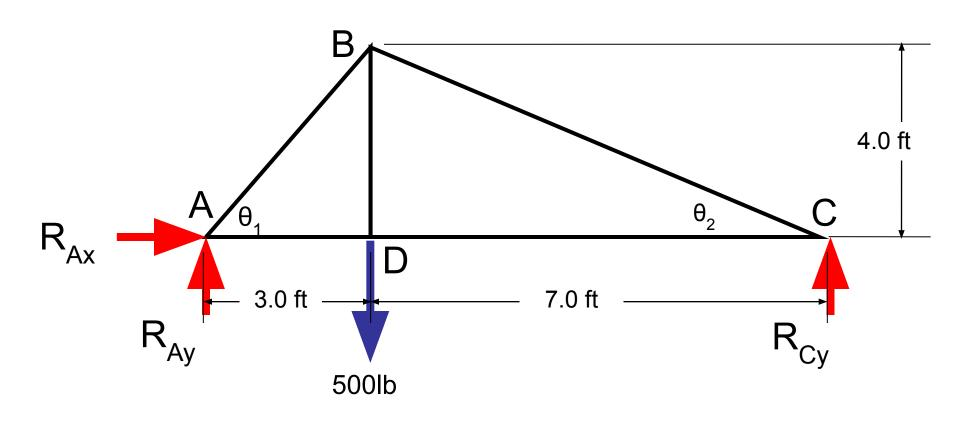
Using Truss Dimensions to Find Angles
