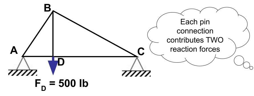
A truss is considered **statically indeterminate** when the static equilibrium equations are not sufficient to find the reactions on that structure. There are simply too many unknowns.
