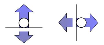
A roller support can support a structure in only one dimension.
